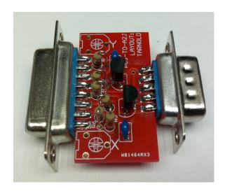
The final parts to install are the trimmers. They just pop in and are soldered in place like everything else. And now its complete. I would center both trimmers so you have a good starting point.
